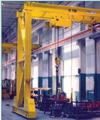
Overhead & Gantry Crane (Lifting)
